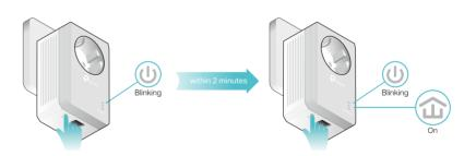
blinking. When the Powerline LED  $\widehat{\mathbf{u}}$  stays on, the pairing
